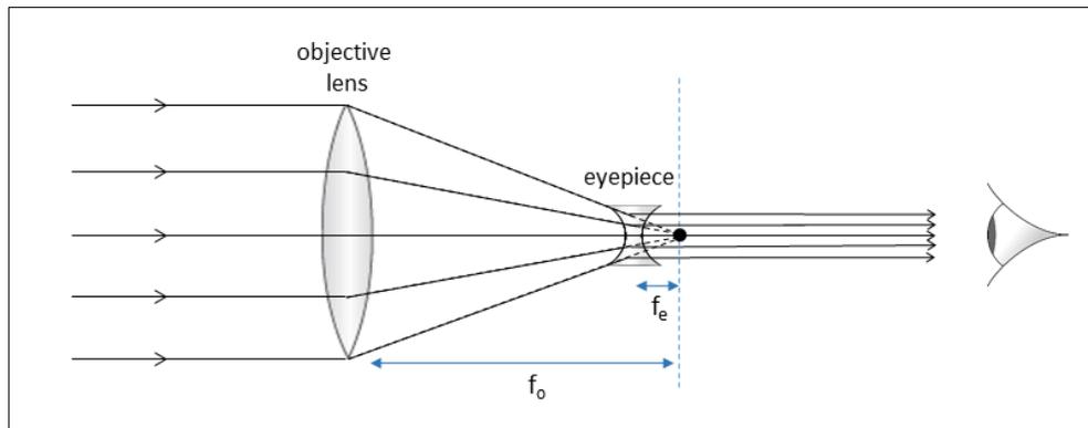
Figure 7: A concave lens as a telescope's eyepiece
