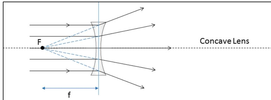
Figure 3: Light paths through a concave lens
