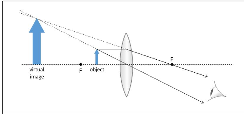
Figure 5: A convex lens as a magnifying glass
