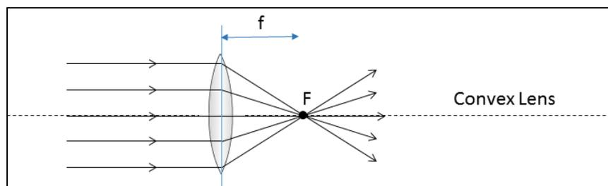
Figure 2: Light paths through a convex lens
