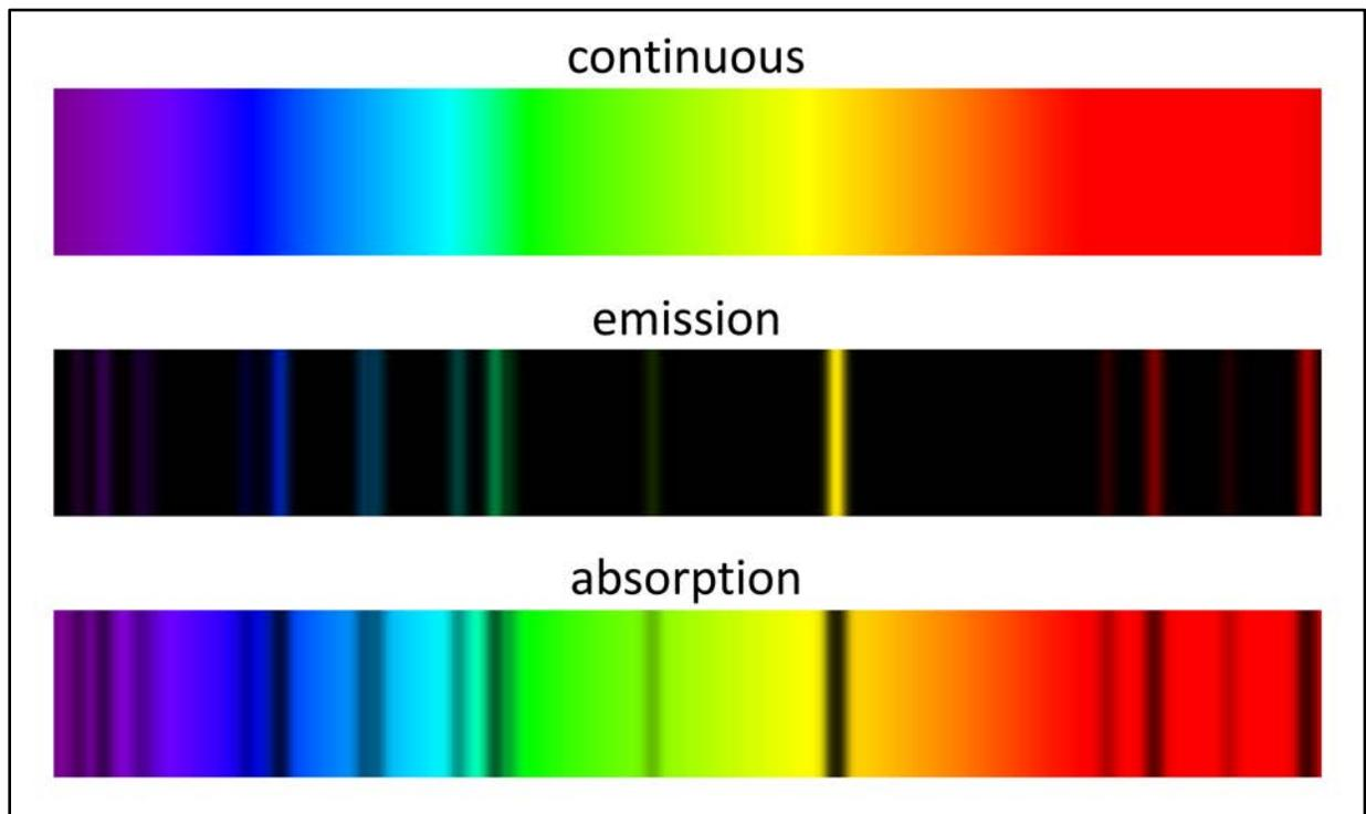
Figure 1: The three types of spectra
