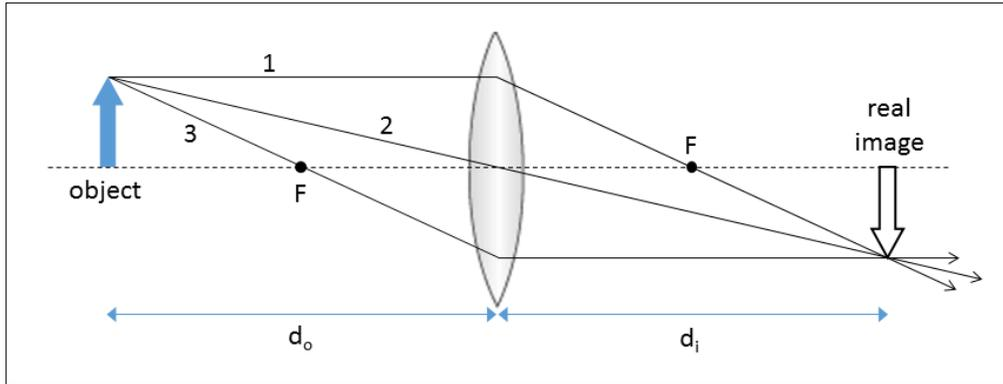
Figure 4: Image formation with a convex lens
