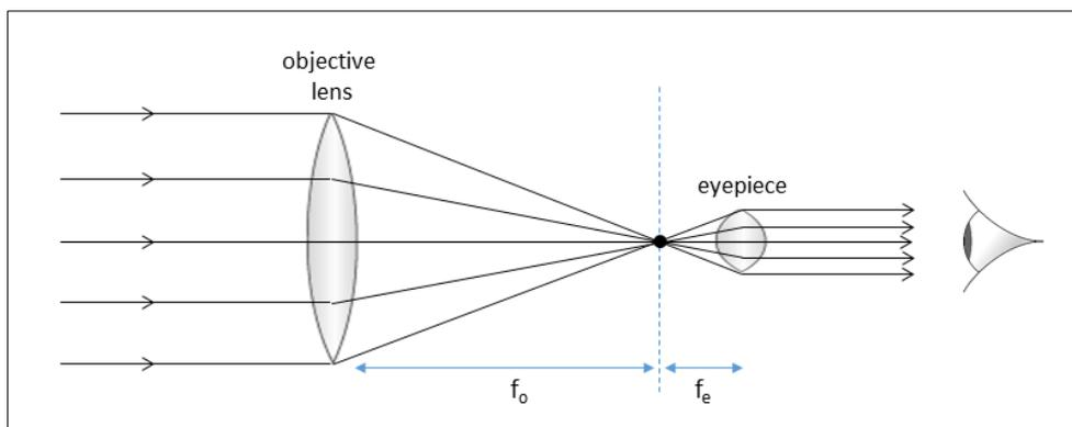
Figure 6: Two convex lenses making a telescope
